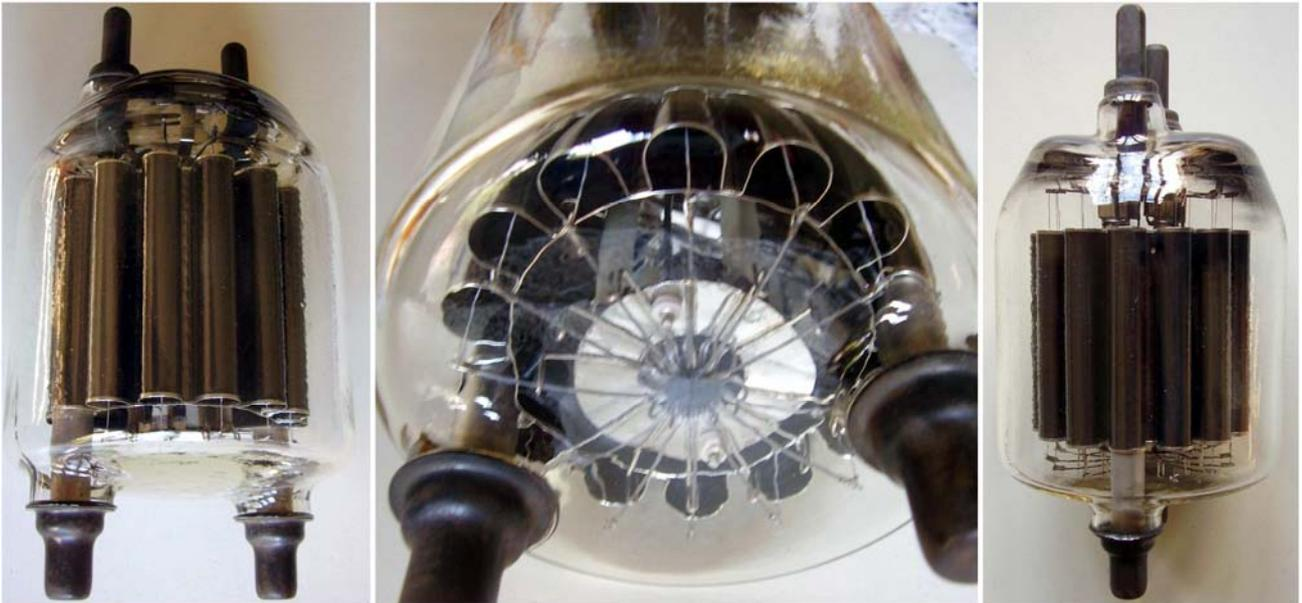
Large rectifier, intended as voltage clipper in radar transmitters.
