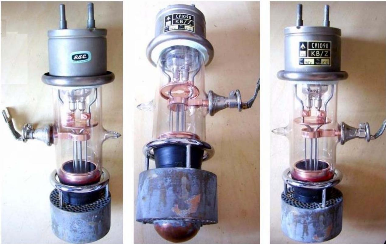
Transmitting triode intended for pulse operation. Heavy copper anode radiator. Thoriated tungsten filament, 750 W anode dissipation with forced-air cooling. Capable of generating 100 kW pulses at 100 MHz, usable up to 250 MHz with reduced power.
