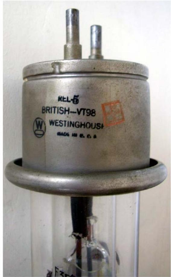
CHL systems were built by Canadian REL and supplied to the United States for the surveillance of the Panama Channel. Transmitting tubes were manufactured by Westinghouse both in America, as for the above sample, and in Canada.
