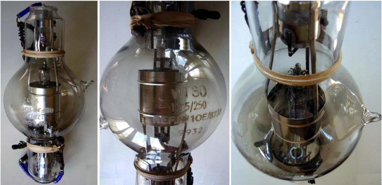
According to Tyne MOV introduced its T250, 250 W transmitting triode, in 1922. This type was accepted by British Post Office as VT30 and by Royal Air Force as 10E/8738. Later different specs were unified in the CV register under the [CV1030](#) title.
