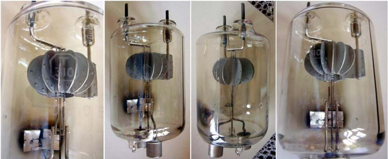
No information found on this Japanese VHF power triode. Arrangement of electrodes recalls the one of German triode [LS180](#), used in the transmitter of Würzburg radar. Grid and anode are terminated to the relatively small pins on the top. The filament terminates into two quite large caps on the bottom. The bulb looks made of hard glass.
