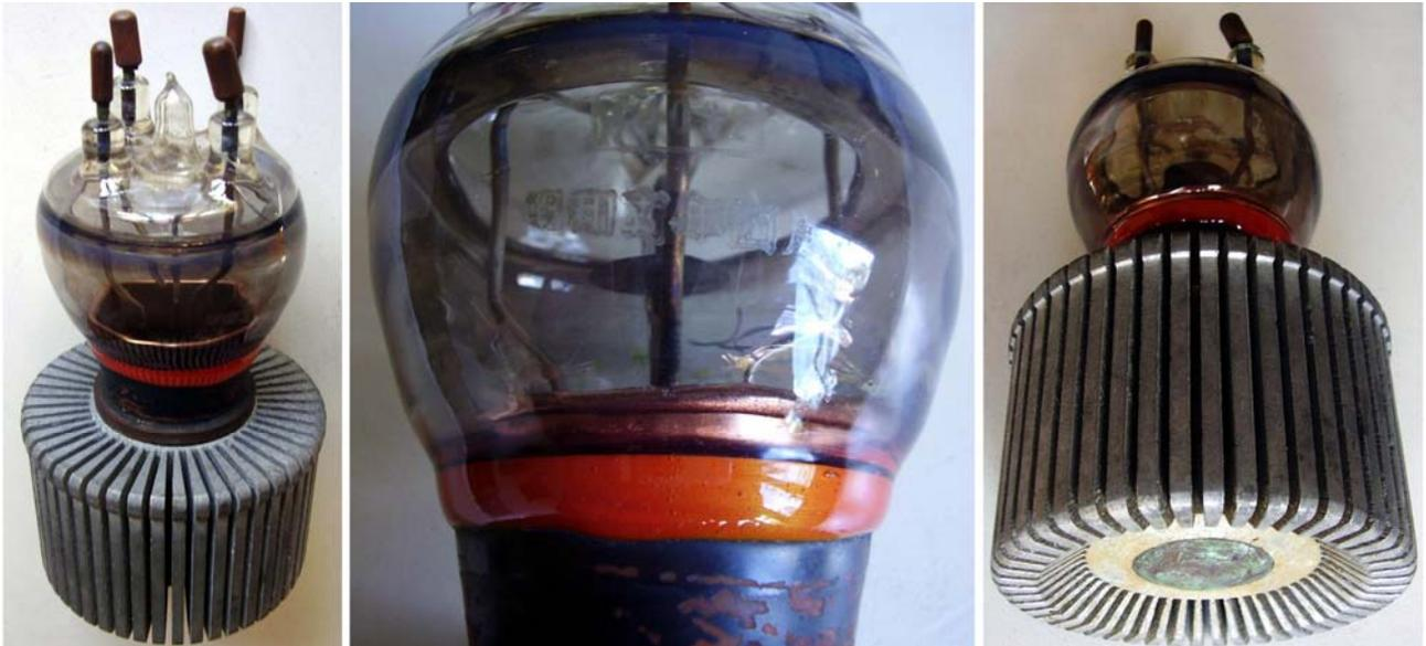
RT-323 is an external anode triode, requiring forced-air cooling to operate at 750 W max anode dissipation. Probably developed by Toshiba for the Army mobile ultra-short warning set Tachi No. 7. The radiator is made of very light material, likely a sort of aluminum alloy. Looking for more information.
