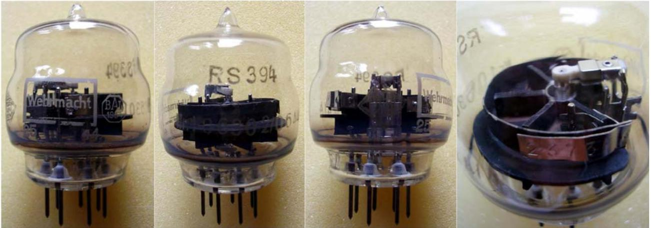
RS394 was designed to operate as power amplifier or oscillator at frequencies up to 560 MHz. Two tubes in push-pull were used in the transmitter of the FuG202 Lichtstein radar since early 1941. Oxide-coated unipotential cathode, finned anode. Later the design was made simpler, to increase the production, originating the variant LS30. RS394 can be seen as the German equivalent of the Eimac **15E**.
