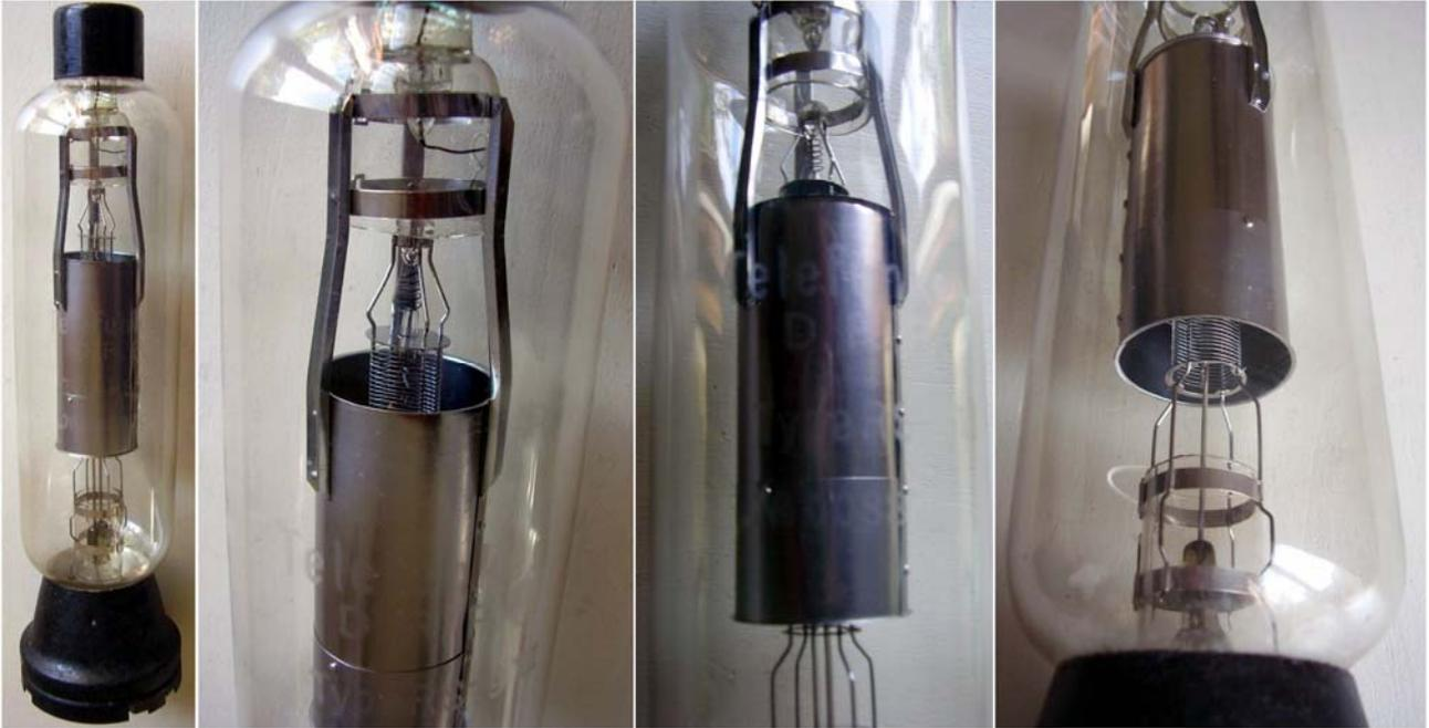
Transmitting power triode introduced by Telefunken in 1919. 235 mm high.
