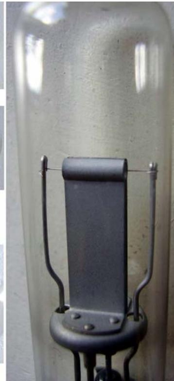
This is an extremely rare sample of split-anode 3 cm CW-like magnetron. It recalls the type described by Kilgore in pages 14 and 15 of his paper (\*1). RM 4025 never went into full production and about 50 units were made before the end of the war.
