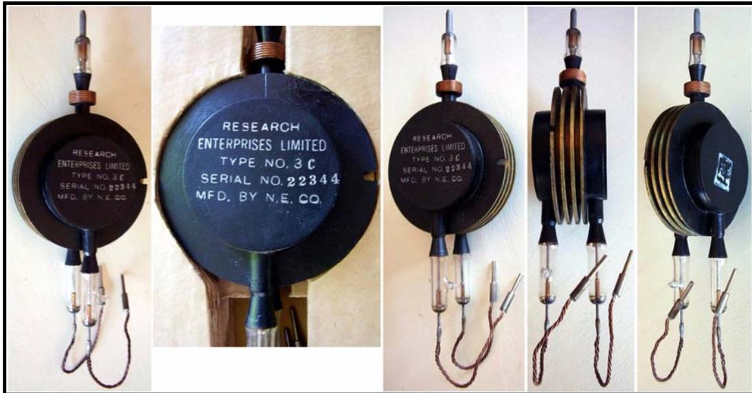
Early cavity magnetron, similar to E-1198 and to [CV38](#).
