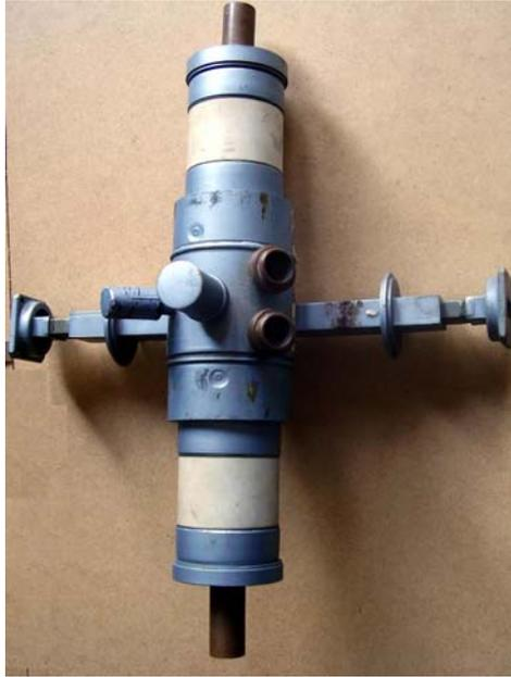
No data found on this Raytheon Amplitron. Based upon the section of the two waveguide sections, it should operate in the X-band. Below the answer from Danial Stocks, TCA:
