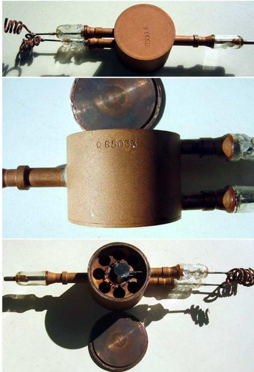
This magnetron is believed to be a 10 cm early developmental sample of the strapped type. Likely built in 1941 at Birmingham by someone from the group of Sayers. Early asymmetrical strapping scheme using only four straps per side. We find the same strapping arrangement in [CV56](#), in [CV76](#) and in its successor [CV1479](#).
