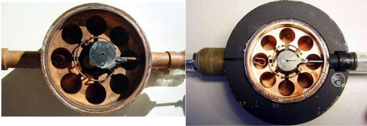
In this image a close-up view of the internal strapping arrangement of our sample compared with the very similar one of a CV1479.
