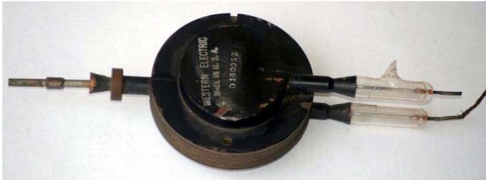
Certainly other qualification copies were made by Raytheon, but their number is not known. Supposedly in the late 1940, being in very short supply copper and other imported materials used in the fabrication of magnetrons, the design was revised. In all the successive productions the original 8-fin copper radiator visible in the above photo was replaced by the 4-fin machined-brass one.
