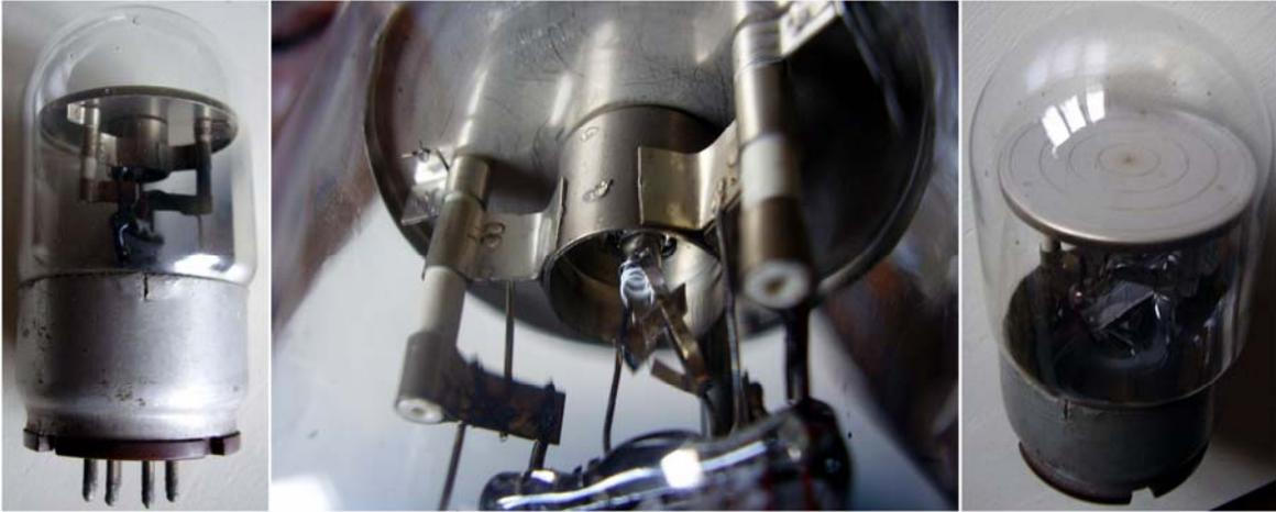
No code or manufacturer can be read on this tube. Nevertheless it closely recalls the cathode ray tube designed by RCA to explore the magnetic field distribution over wide spaces. This device was described in [Electronics, July 1938](#).
