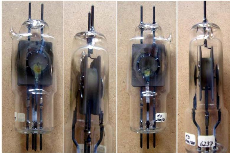
This is an undocumented 'Turbator' magnetron by Brown Boveri. According to its code it can give in output 500 W at 2.400 MHz.
