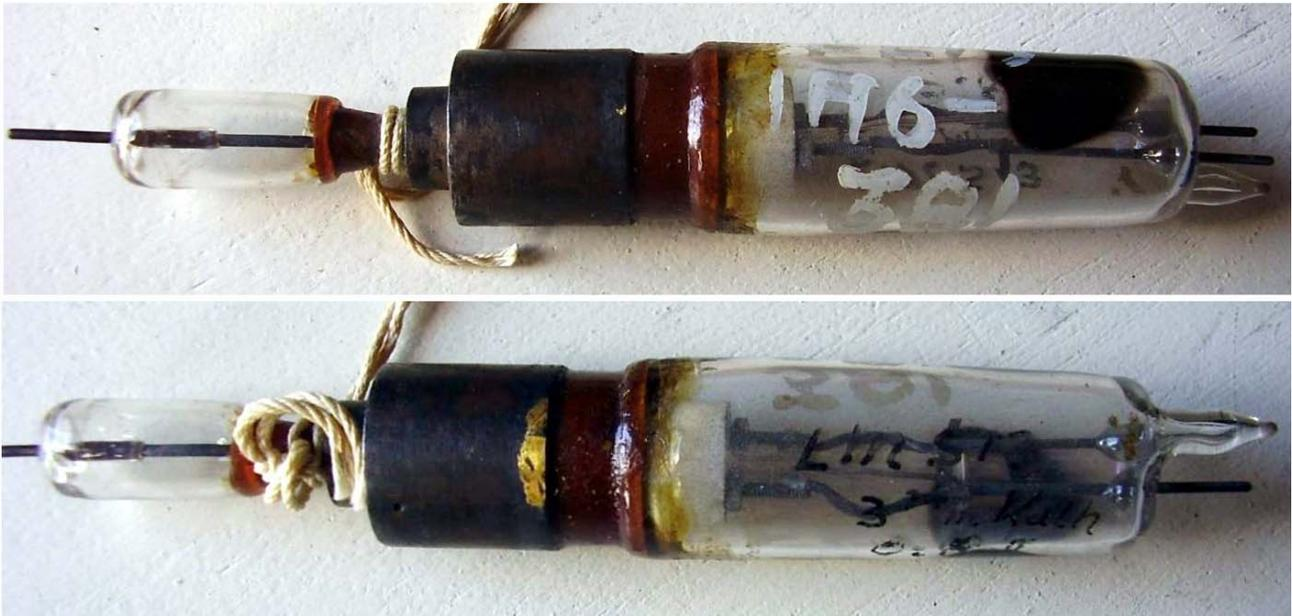
LMS 13 was just in a quasi-prototypal sampling stage when the war ended. In the table below we learn that about ten units per month were being made. Similar to LMS 12 but much smaller, it measures approximately 120 mm length by 20 mm diameter.
