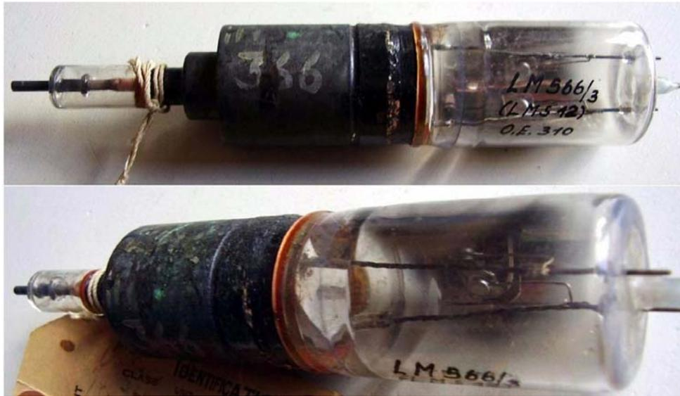
LMS12 was one of the few multicavity magnetrons to go in production in Germany before the end of the war. Its use was anyway limited to a few tens of airborne equipment operating at 3 cm, as the Bremen FuG244 also known as Berlin D, and to some experimental sets. Its shape departs considerably from that of LMS10, the first 10 cm multi-cavity magnetron copied from the British CV64.
