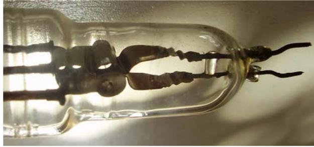
**Fig. 5 - Close-up view of the internal resonating line strip, connected to the outside by means of wavy sections rigidly interlocked by a glass spacer on the right**
