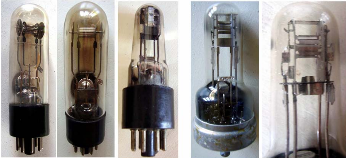
Fig. 1 - Experimental samples of 8 and 12-segment 'squirrel cage' magnetrons built at GEC in the development of the two tubes shown on the right, the E1429-CV79 and of the E1430-CV89.
