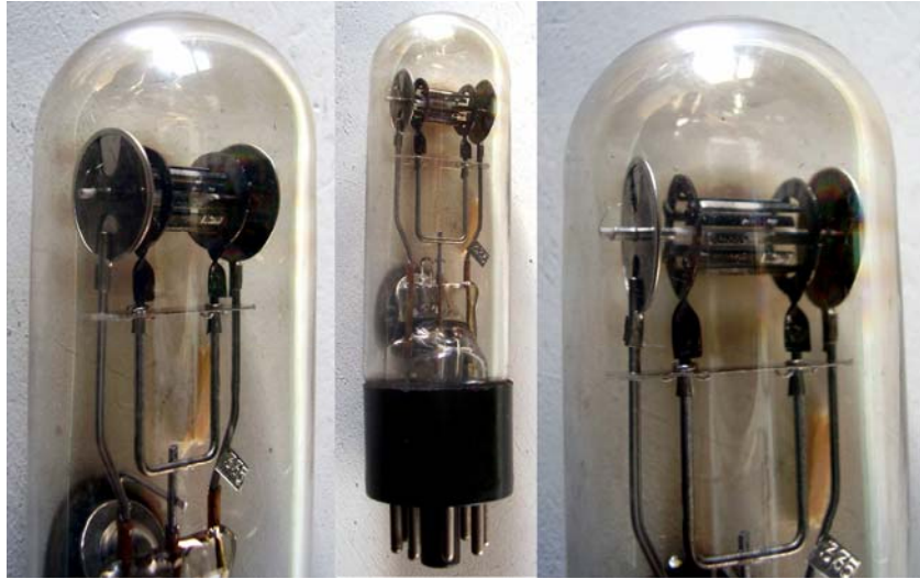
Fig. 2 - 12-segment 'squirrel cage' laboratory prototype.
