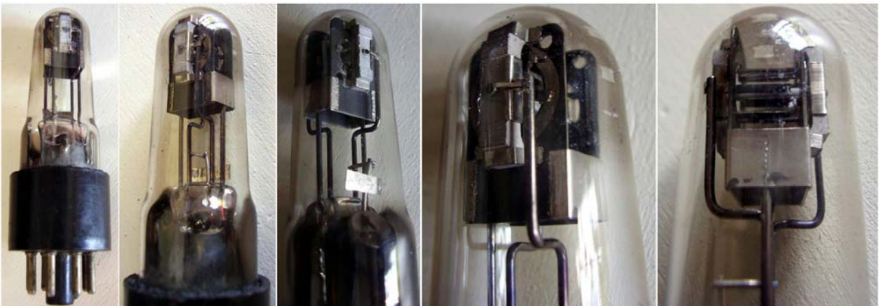
Fig. 4 - The third sample looks almost definitive. If we exclude the octal bakelite base, the glass bulb appears tapered and the electrodes are enclosed in a boxed structure.
