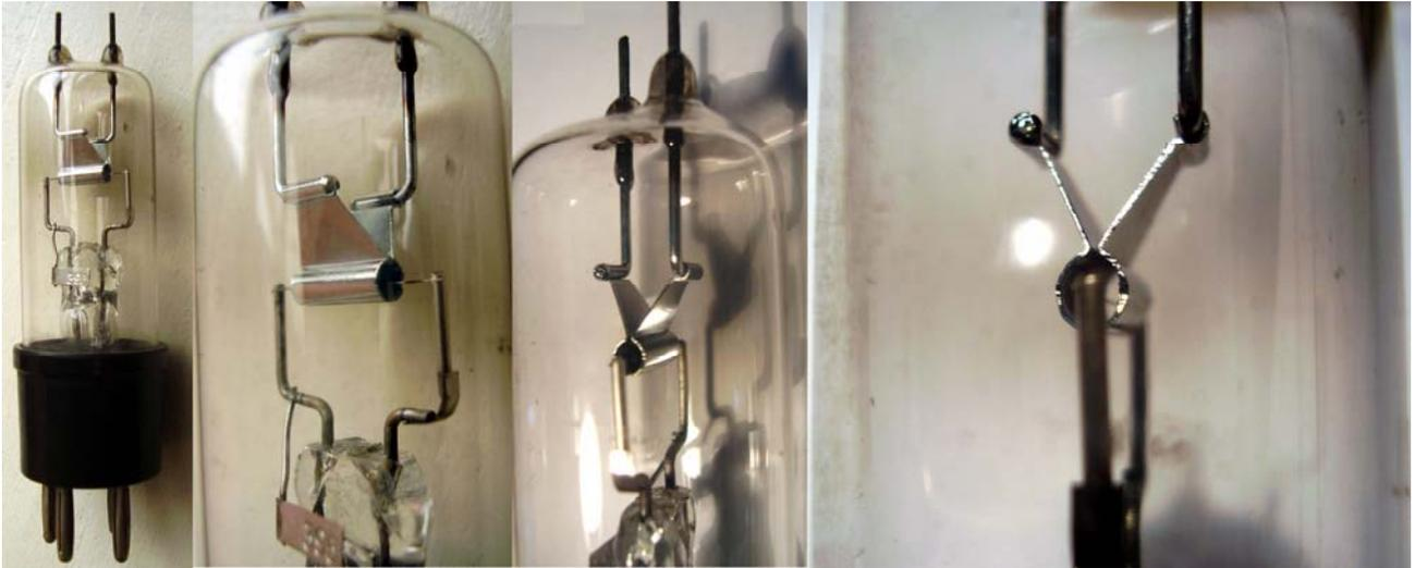
This magnetron is quite small, about 100 mm high by 25 mm diameter. The anode split cylinder measures about 10 mm by 2 mm, tapered ends welded to the L-shaped top pins. The filament looks very tiny, 0.1 mm diameter or so. A number 395 is stamped on a small label in the bulb nearby the glass press. The construction appears simple but very clean, sturdy and accurate.
