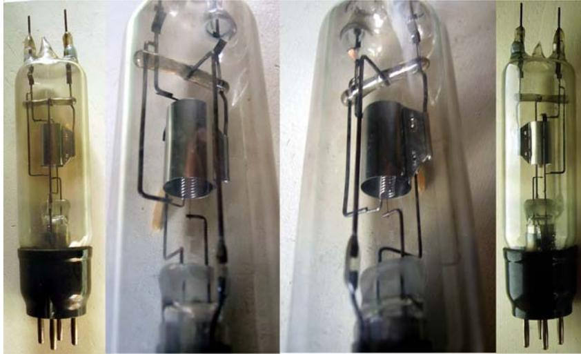
Probably this sample is what today survives of the Megaw's early experiments on CW cylindrical magnetrons with built-in grid, to directly modulate the RF output signal.
