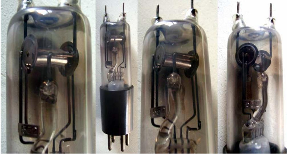
The GEC experimental split-anode magnetron No. 2 is quite small. It is about 11 cm high and the glass bulb diameter measures about 23 mm. 4-pin midget base. The code 552 is punched on a small tsg inside. Anodes form a cylinder of approximately 10 mm by 5 mm in diameter. The two cylinder halves are supported by rods that enter from the top of the bulb and end on the top of two molded glass stems anchored near the bottom pinch. The interaction space is delimited by two end plates.
