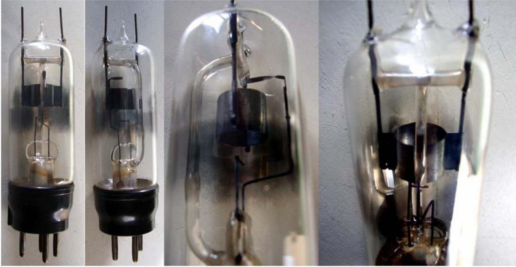
This sample of GEC split-anode magnetron looks very early, with its vertical electrode structure anchored to a molded complex glass frame. The same ratio between the considerable diameter of the anodes and their reduced height suggests a construction before 1935.
