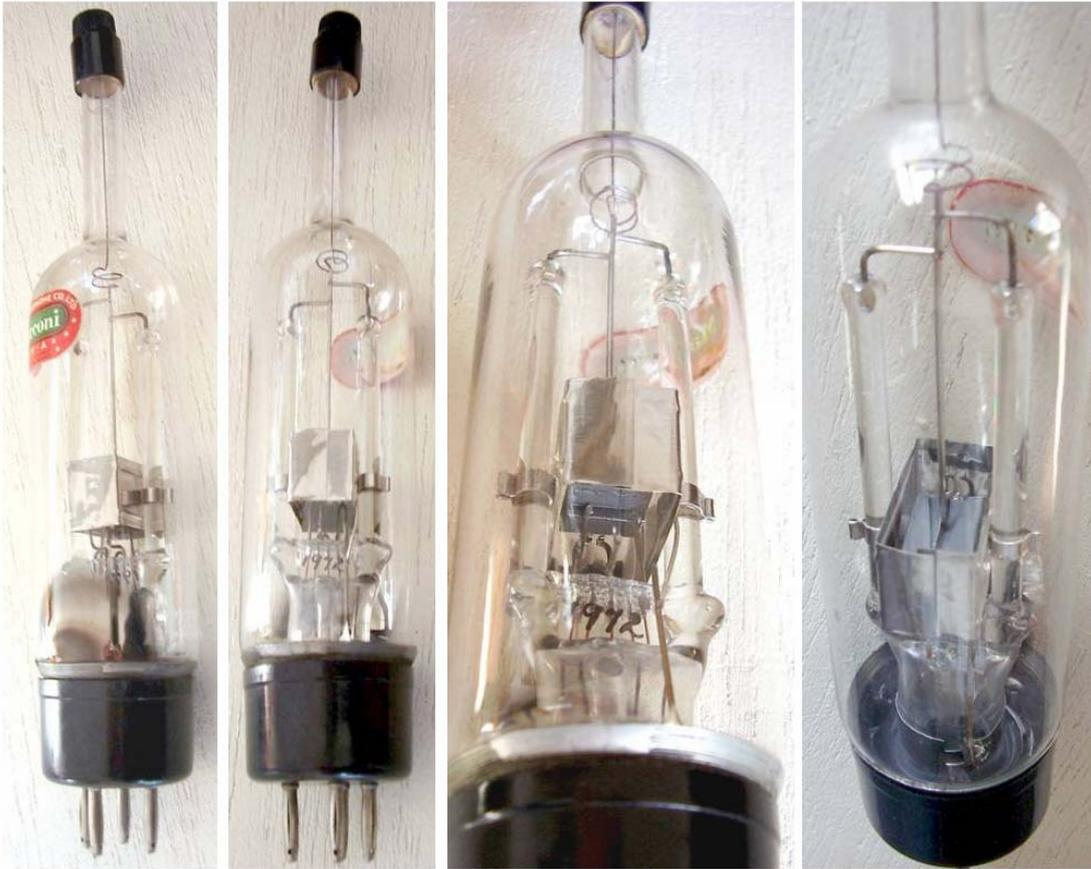
Electrometer triode for high impedance measurements. The grid is connected on the top of the high glass stem. Introduced between 1936 and 1937.
