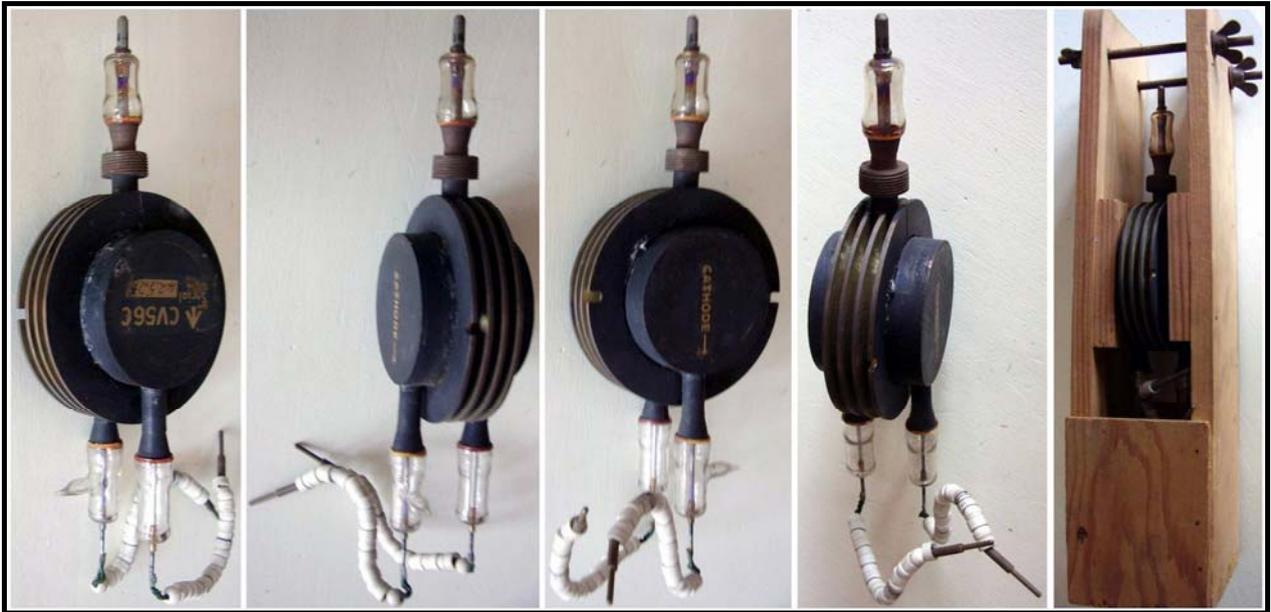
CV56C was derived from [CV56](#), bending the straps in order to make each unit to oscillate at one of the four different frequency variants, identified by the suffix A to D. The frequency variants were introduced to prevent interference between different sets.
