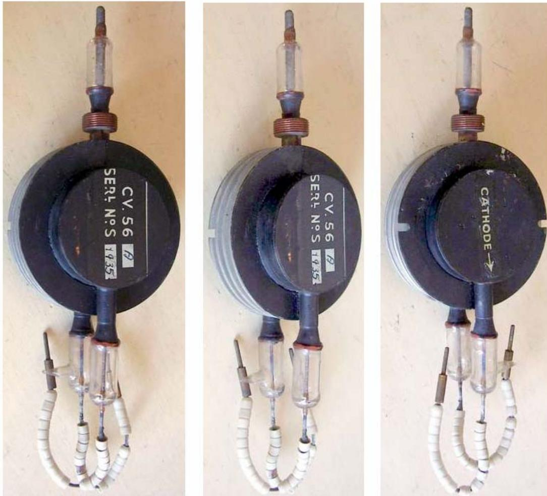
CV56A was derived from [CV56](#), bending the straps in order to make each unit to oscillate at one of the four different frequency variants, identified by the suffix A to D. The frequency variants were introduced to prevent interference between different sets.
