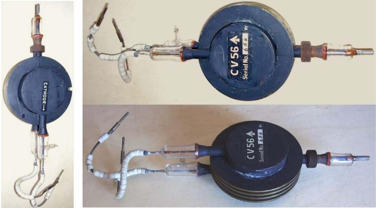
CV56 was derived by the very early unstrapped 8-cavity magnetron NT98, adding strap jumpers to prevent unwanted modes. The strapping developmental work was run at Cambridge by Sayers. The [Q85033](#) is one experimental sample with the same asymmetrical strapping scheme. CV56 was the first strapped magnetron to enter into production around the late 1941. Soon replaced by four frequency variants, including [CV56A](#), [CV56B](#) and [CV56C](#).
