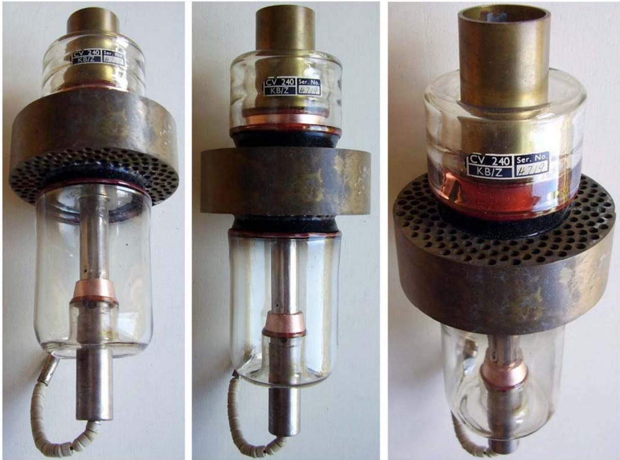
This is the largest micropup triode. It was designed by GEC, developmental code E1495, for high-power pulse applications in the VHF spectrum up to 100 MHz. Design started in April 1944 leading to a preproduction around the end of the year.
