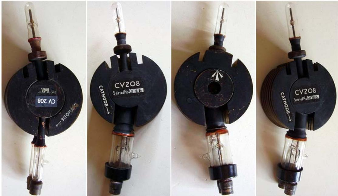
E1487, approved as CV208, was the first GEC X-band 12-segment double ring strapped magnetron. The collection includes the very rare early double stem release, left, and the single stem production release, the latter fully compatible with the BTH [CV209](#).
