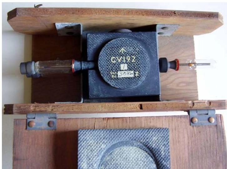
Below, construction details of the CV192. Quite interesting the handcrafted glass spacers, which firmly hold the output probe, preventing harmful vibrations.
