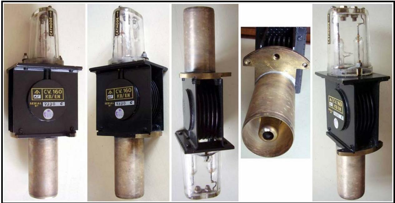
S-band strapped magnetron. One of the few British magnetrons provided with glass boot supporting heater and cathode connections. Coaxial output, external magnet. The tube was developed early in 1944 for use in high-power ground radar, being capable of handling up to 1 MW input pulses.
