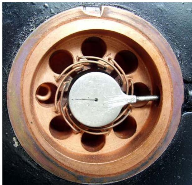
Close-up view of the echelon strapping used in CV160 magnetron to prevent oscillations in other than  $\pi$  mode.
