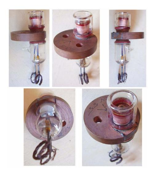
UHF milli-micropup transmitting triode. Conduction-cooled through the copper anode brazed radiator. Forced air cooling on the grid seal may be required.
