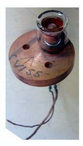
UHF 'milli-micropup' power triode. Milli-micropup power triodes were introduced early in 1941 by GEC as evolution of micropup triodes, <u>VT90</u> or <u>NT99</u>, to operate at frequencies as high as 1200 MHz. Derived from the E1190 GEC design, CV155 was tested and specified for pulse operation up to 1200 MHz. Similar to <u>CV55</u>, this one rated for CW operation, and to the high gain variant <u>CV178</u>.
