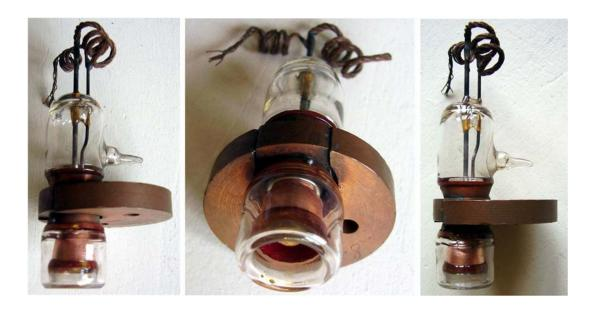
Service code for E1458 GEC milli-micropup transmitting triode. High gain variant of CV155, intended both for CW and for pulsed operation up to 1200 MHz. See also National Union 3C27.
