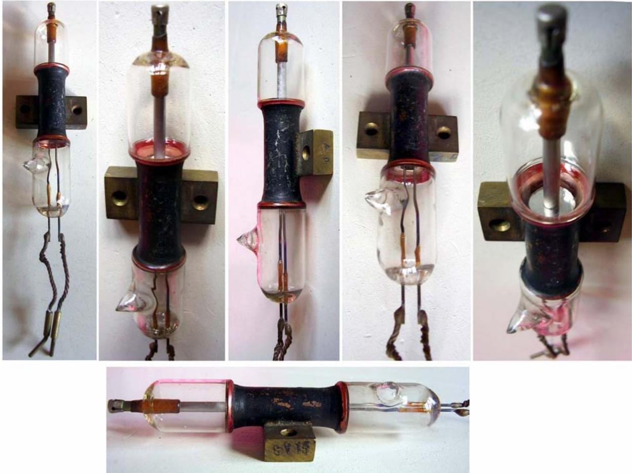
CV15, GEC prototype E.1266, is an external anode VHF power triode. It is a conduction-cooled triode, reduced power variant of the early micropup [VT90](#). A couple of CV15s in push-pull produced 10 kw pulses, 1  $\mu$ s at 1500 pps in the 70 cm ASV airborne radar. Later replaced by [NT99](#). Cooling must be provided by suitable radiator so that anode temperature does not exceed 140°C.
