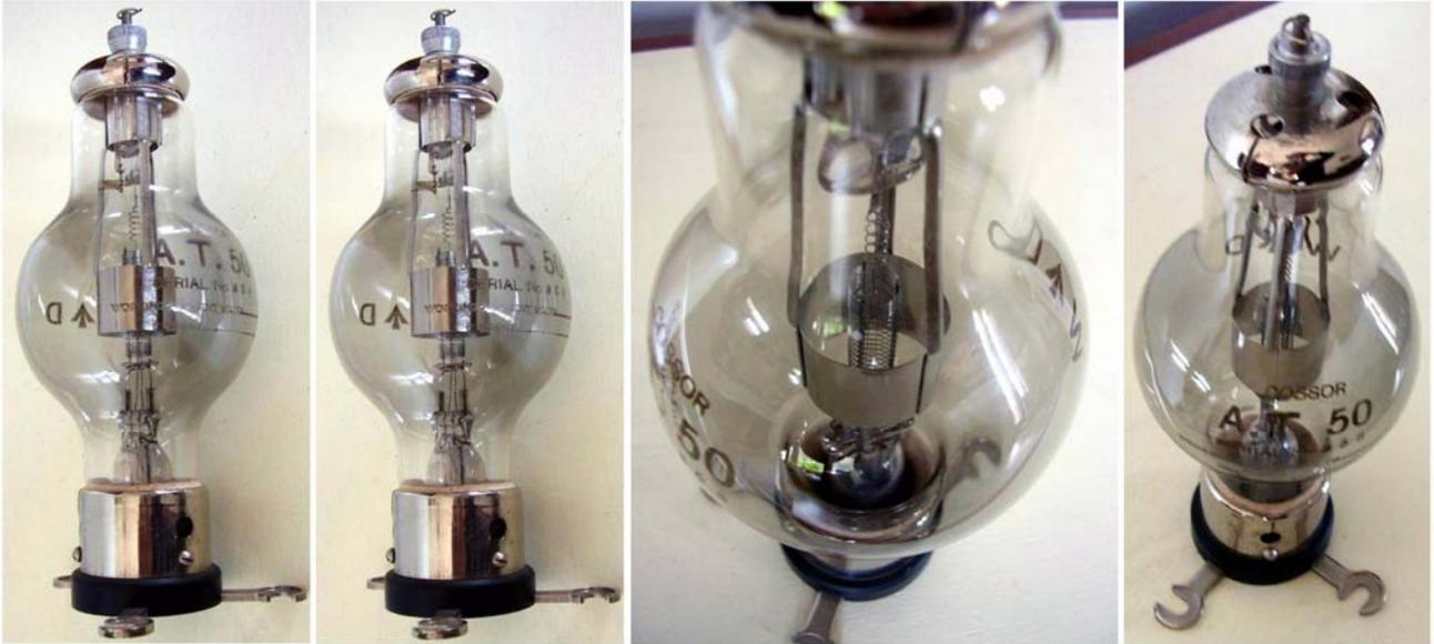
50 watt transmitting tube made for the British Army by MOV, Edison-Swan, BTH and A.C.Cossor Ltd.
