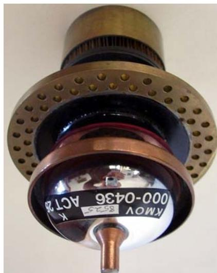
Actually the cap corresponds to heater, followed by a heater-cathode ring, by the drilled grid disc and by the finned anode radiator.
