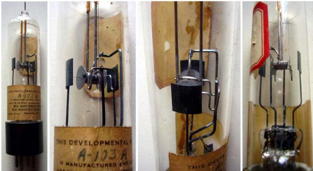
This looks to be a split-anode magnetron with self-contained resonating line terminating loop. The two anode half cylinders are connected to the two top pins. The connecting rods are shorted together shortly above the anode, likely to form part of the resonating system. The position of the shorting rod suggests that the tube was designed to oscillate at very high frequency and indeed the data sheet of the 2J35 gives 10 cm approximate wavelength.
