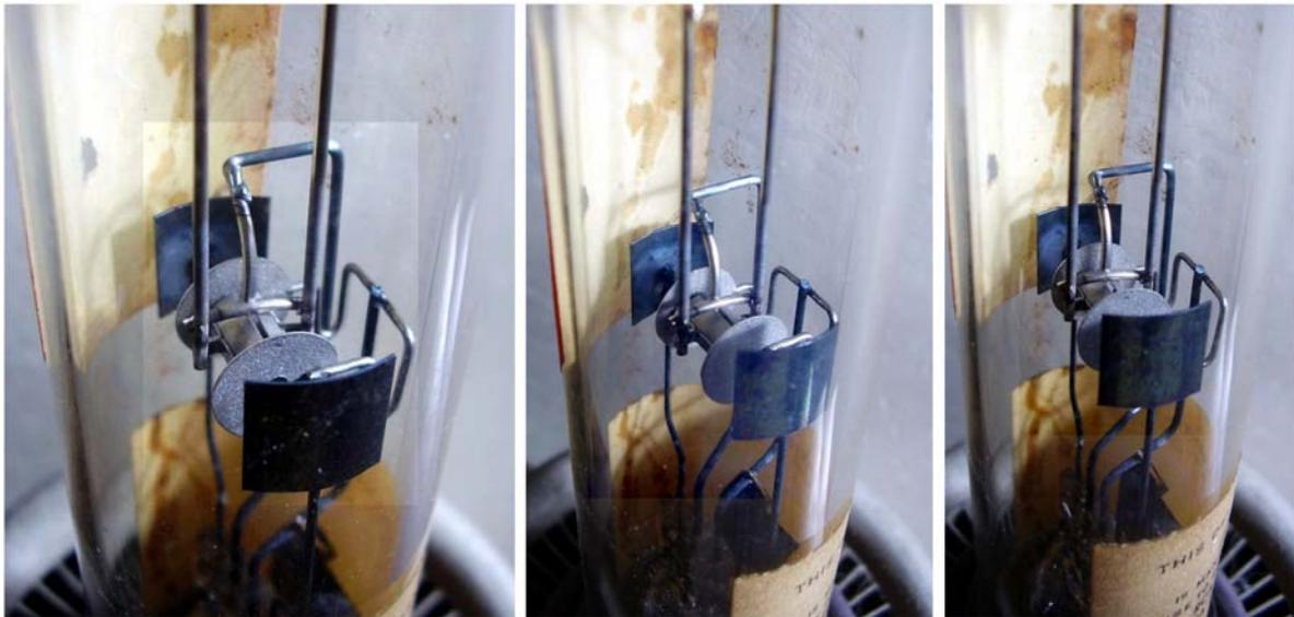
Here are some close-up views of the resonator formed by two vertical segments, about 5 mm each, and the two halves of the horizontal shorting jumper. The center of the jumper is connected to one pin of the base. The equivalent line is about 1 cm long and should resonate at about 4 cm.
