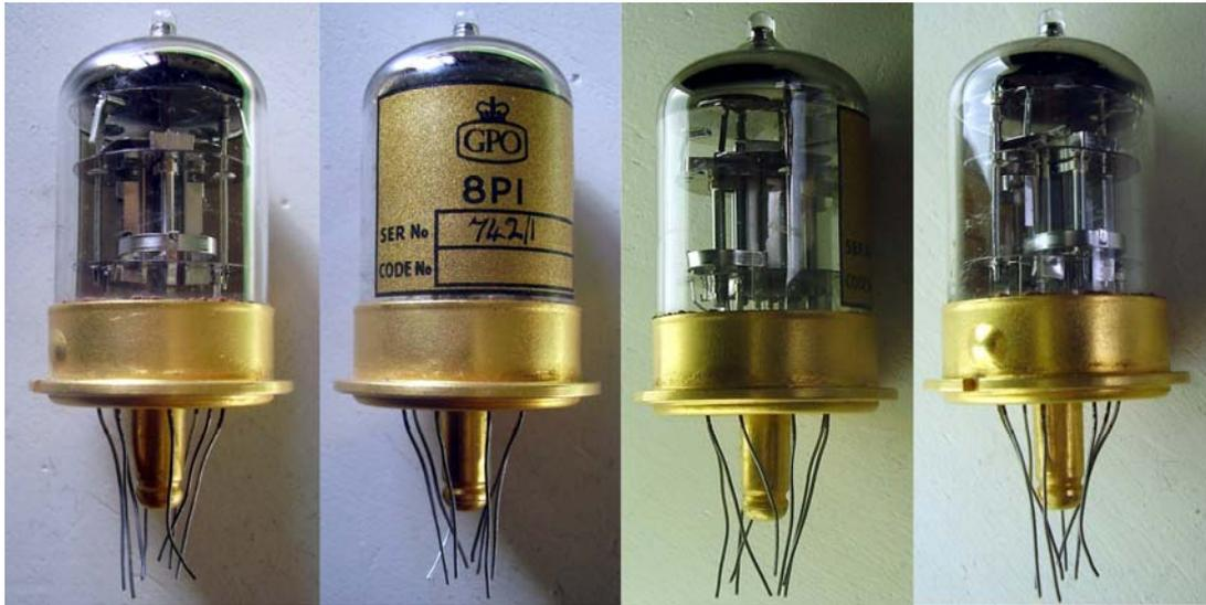
Ultra reliable pentode designed as low-voltage, high-transconductance amplifier for submarine telephone repeaters. The article describing the family of low-voltage tubes appeared in 1962 in the paper 1890 from The Institution of Electrical Engineers.
