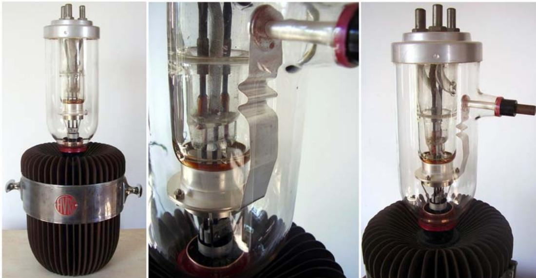
Here is a huge transmitting triode derived from the water-cooled 891 type with the addition of a big finned radiator. 559 mm high, 206 mm dia, 20.4 kg net weight.
