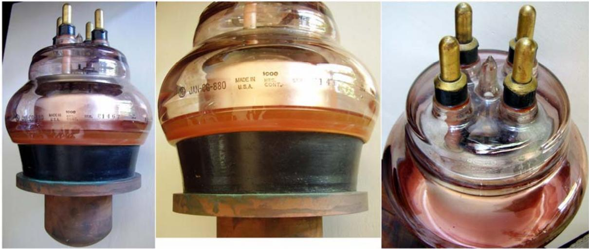
External anode, water cooled transmitting triode, capable of dissipate 20 kW anode power. The introverted anode makes it possible to minimize the inductance and the overall tube height. The tube is intended for radio or industrial applications, for frequencies up to 25 MHz full ratings. Pure tungsten filamentary cathode.
