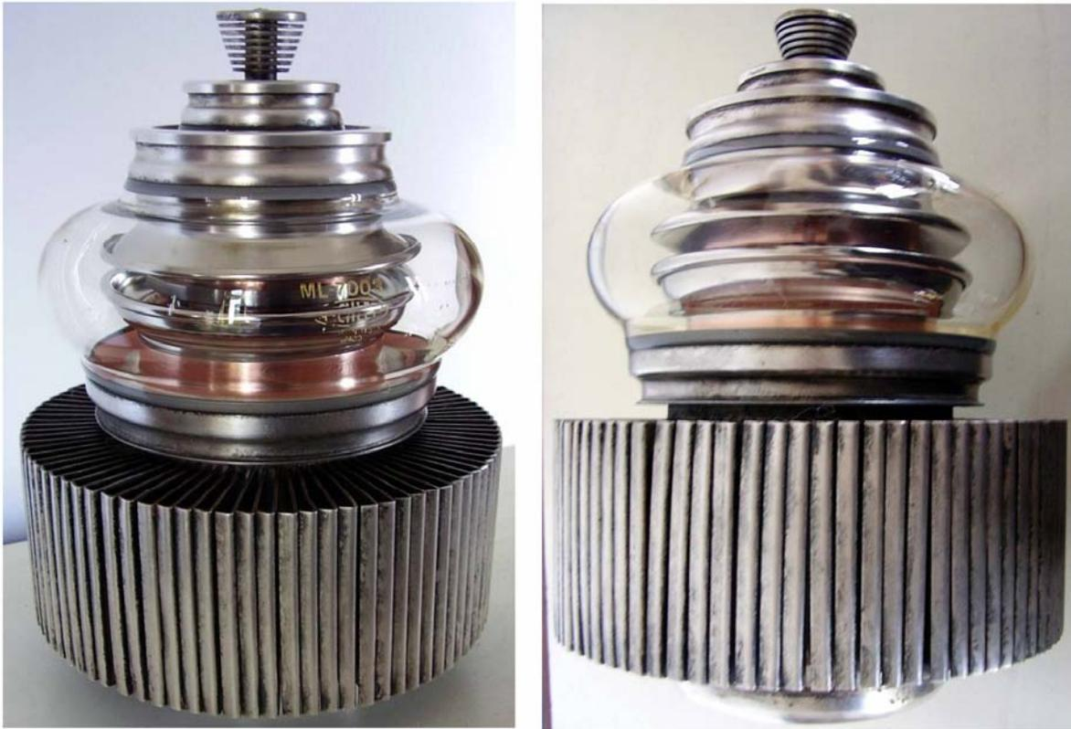
Screened-grid high-power triode intended to operate as switch in hard-tube pulse modulators up to 2 megawatts. 25 lbs, about 12 kg net weight.
