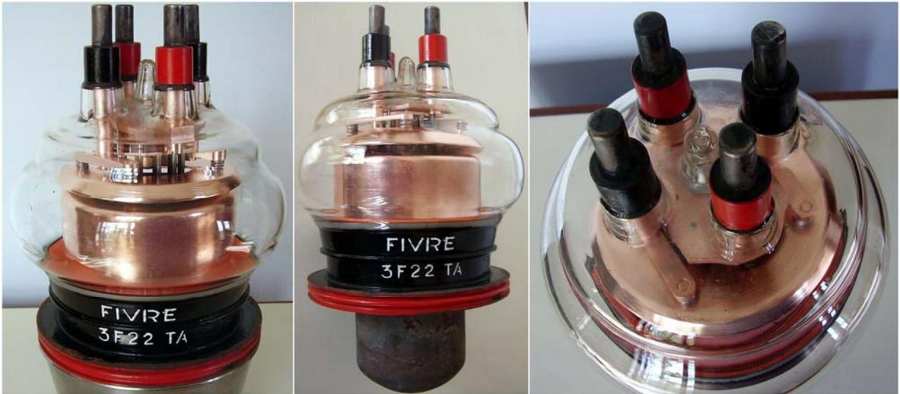
Water-cooled and forced-air-cooled transmitting triode. Similar to [3F20-TA](#) but with folded anode and higher frequency limits. Thoriated-tungsten filamentary cathode. This Fivre code is equivalent to the industry standard **5771**. Also equivalent to Machlett ML-356.
