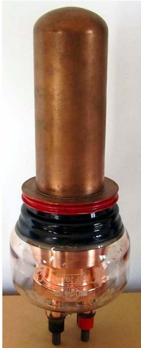
External anode, water cooled transmitting triode, capable of 22 kW anode power dissipation. The tube is intended for radio or industrial applications, for frequencies up to 30 MHz. Thoriated tungsten, direct heating cathode.
