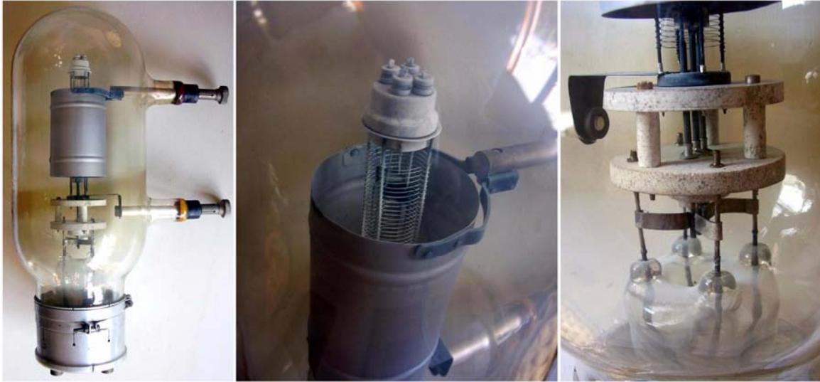
3B600 was made by Italian Fivre. This shape was quite common for RF high-power tubes intended for electro-medical or RF heating equipment. The tube had to be sturdy enough to operate with mismatched loads. Tungsten filamentary cathode.
