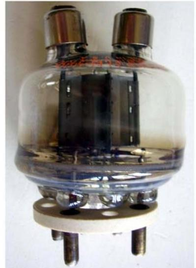
High-mu VHF power triode, hard glass body with 5-pin ceramic dish base. Plate is supported by two rods terminating in two top caps. It can be considered a compact variant of 356A power triode, intended for operation up to 150 MHz full ratings and up to 300 MHz at reduced ratings.
