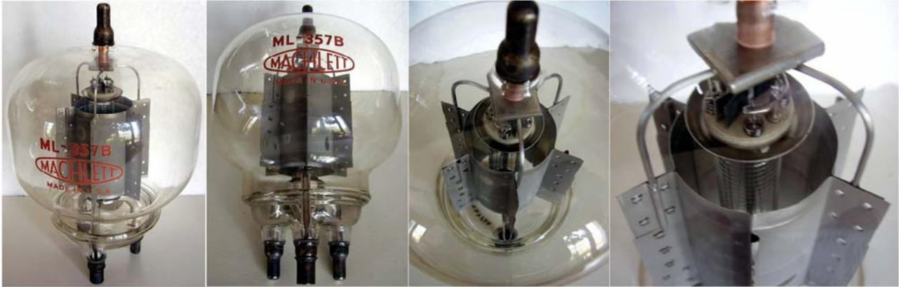
Transmitting power triode capable of operation in the VHF region. All glass body. Forced-air cooling required when operated full-power above 40 MHz. Thoriated tungsten filament.
