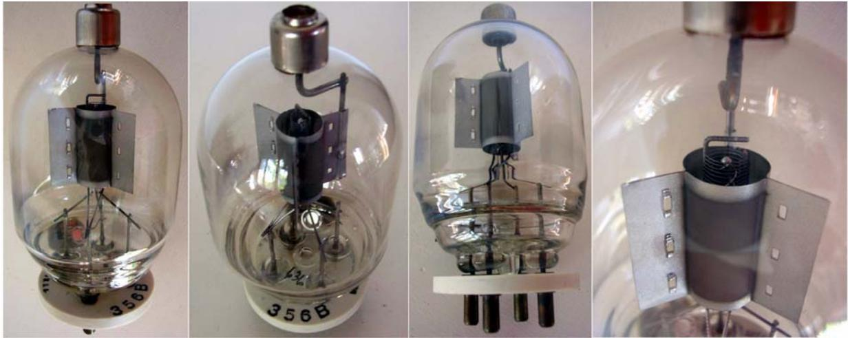
Few info found about the origin of its parent **356A**. The tube was introduced by Western Electric between 1938 and 1939 as improved 100-TH, then used as early radar pulse modulator. Six 356A's replaced a group of six 100-TH's in the pulse modulator of the CXAS and Mark 1 naval radar sets. Prototypes were known with their developmental code D-159781. All-glass T-18 bulb. Top cap and 4-pin ceramic-dish base. Thoriated-tungsten center-tapped filament.
