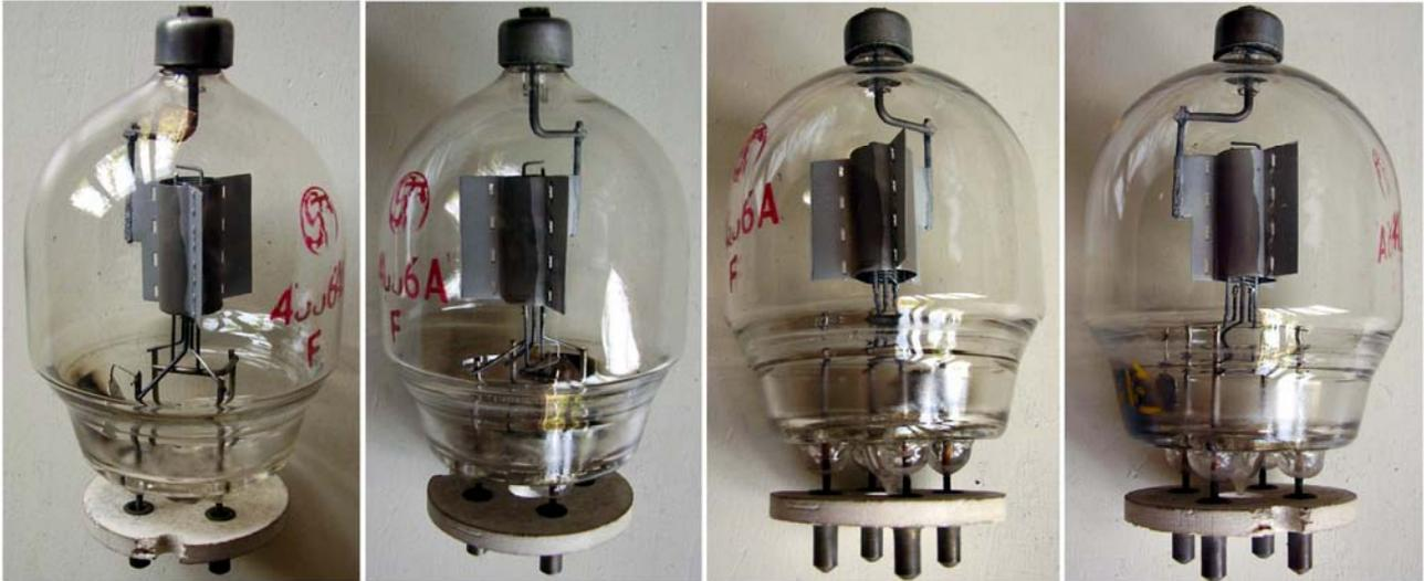
356A was introduced by Western Electric between 1938 and 1939 as HF / VHF transmitting triode. The tube was also used as early radar pulse modulator. Six 356A's replaced a group of six **100-TH**'s in the pulse modulator of the CXAS and Mark 1 naval radar sets. Prototypes were known with their developmental code D-159781. All-glass T-18 bulb. Top cap and 4-pin ceramic-dish base. Thoriated-tungsten center-tapped filament.
