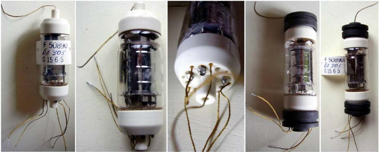
‘On the ocean floor...life begins at 5000 hours’ says a Bell Telephone ad in [Electronics, August 1955](#). This tube was so special that its life could start only after 5000 hours ageing full ratings, equivalent to the whole span life of a high-rel tube or to five average lives of a common receiving tube.
