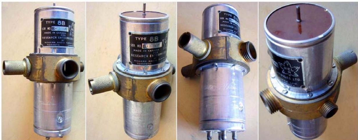
Photos of the REL 8B reflex klystron, directly derived from the Sutton tube, with external shield and semi-fixed tuner, factory-tuned to prevent mode jumping.
