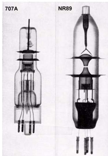
**Fig. 2 - In this image we see on the left the X-ray section of a WE 707A near the section of an early British design. Note the similarities of the 707A, in particular the re-entrant shape of the lower copper disc intended to minimize stray capacitance in the resonating circuit, with the sketch of fig. 1.**
