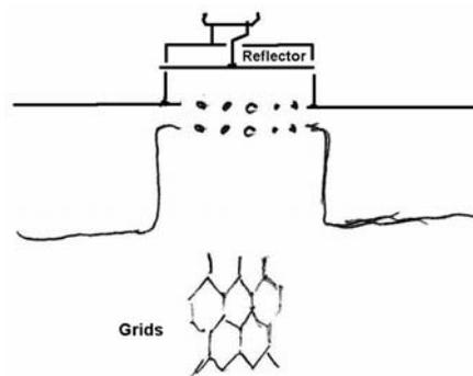
**Fig. 1 - Approximate sketch of the disc seal grids and of the resonator. Looking from the outside, the grids that end the internal extensions of the resonator show a honeycomb structure.**
