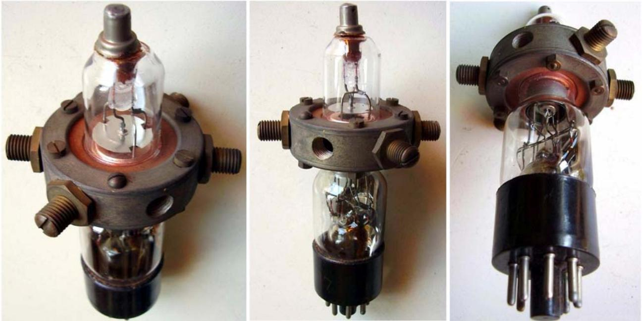
The above sample has no ink markings but the inscription 10AL1, hand engraved on the base with a sharp tip. At a first glance its shape and size could resemble the WE 707A. Carefully looking at its internal construction, some differences can be appreciated. The two copper discs, clamped outside to the external resonator, terminate internally in two gridded flat surfaces, as in the image below. The reflector is a flat dish, probably made of nickel.
