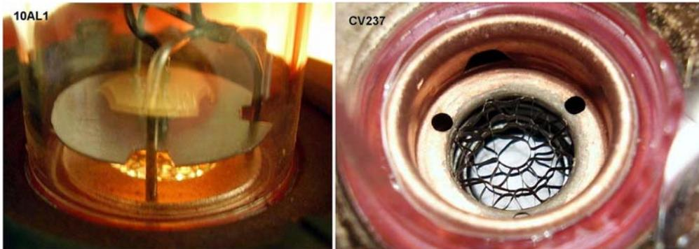
Fig. 3 - Left, a glimpse of the grid meshes in the resonator inner hole of the 10AL1. Right, the ribbon meshes brazed to the inner holes of the resonator discs in a CV237 S-band low-voltage klystron.
