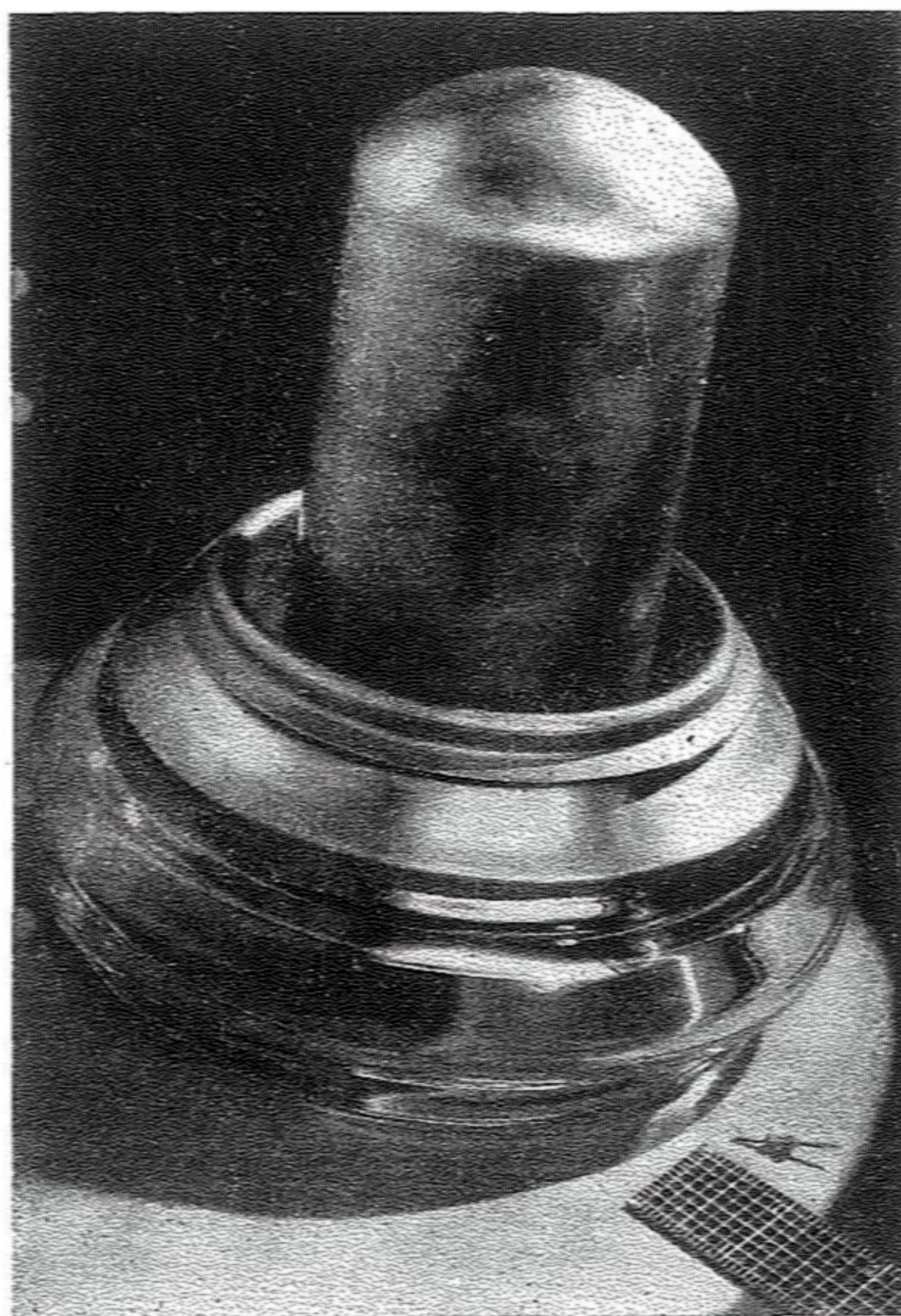
Fig. 18. — Copper anode with Kovar skirt sealed to glass.
