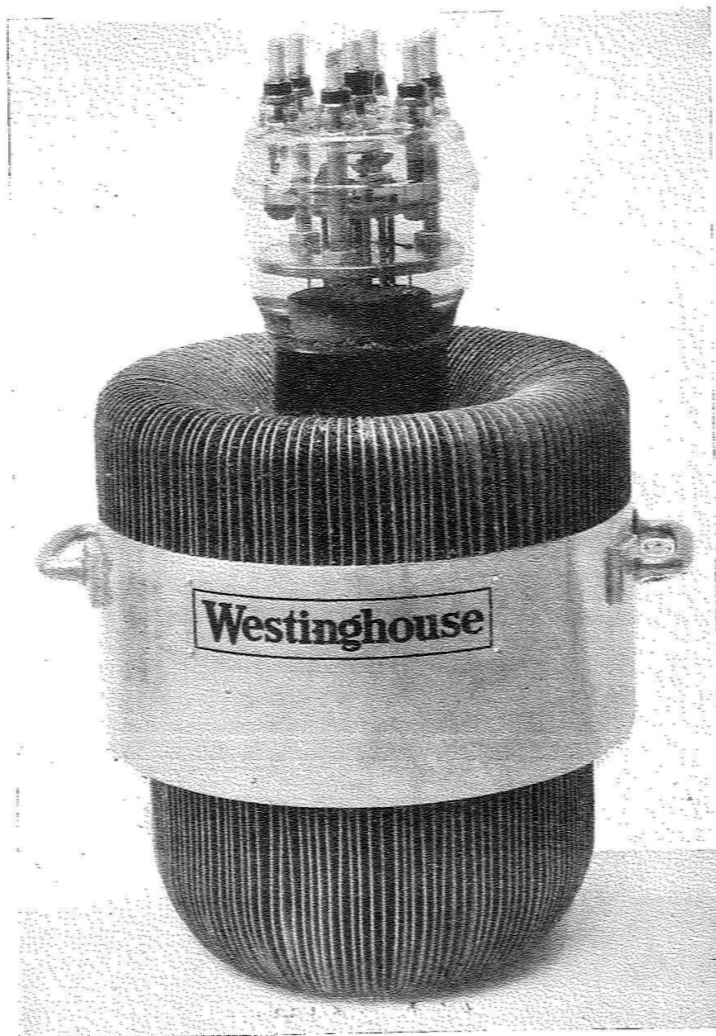
Fig. 6 a. — A modern 100 kW tube (WL-895 type) used in several American broadcast transmitters and in many « tin reflowing » industrial installations. The tube is shown soldered into a multi-fin air-cooler, but can be inserted into a water-jacket instead.
