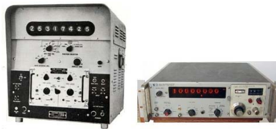
Fig. 14 - The Lavoie LA-80 digital counter on the left and on its right the HP 5245L, here with the HP 5257 transfer oscillator plug-in.
