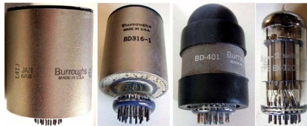
Fig. 6 - From left, the shielded BD-301/6703, the more slim BD316, the BD-401 noise generator and its smaller successor BX-1203/6713.
