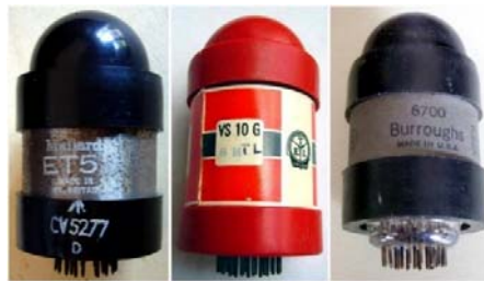
Fig. 9 - The Mullard ET51 and the ETL VS10G compared with the Burroughs 6700.
