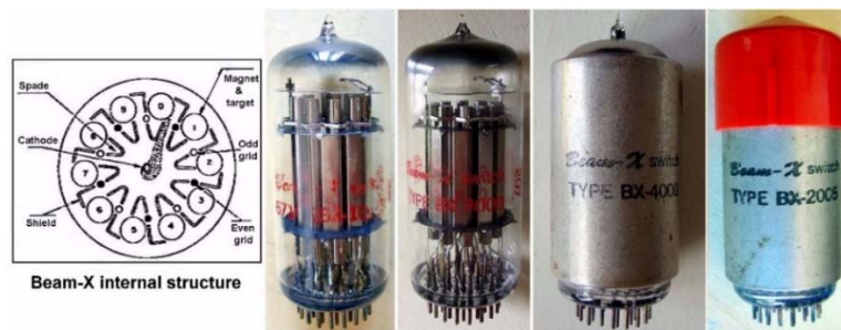
Fig. 8 - Beam-X counters. From left, cross section of the family, the 6710/BX-1000, the high-current BX-3000 and two shielded types, the BX-4000 and the BX-2005.
