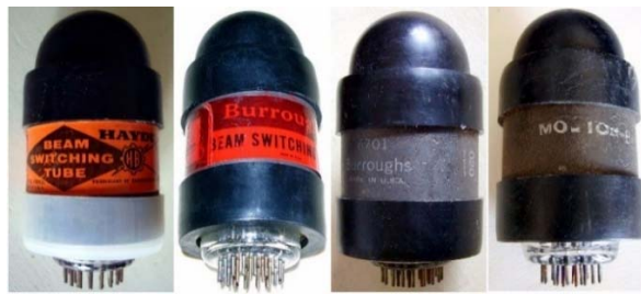
Fig. 5 - From left, an early Haydu badged 6700 tube, a later sample with Burroughs label, a low-voltage 6701 and the high-speed MO-10R/6704.
