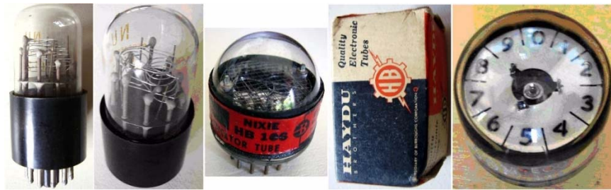
Fig. 10 - Two images of the National Union GI-21 Inditron™, the Haydu-badged HB-106 Nixie™ beside its box and the Amperex/Philips Z550M Pixie™ numeric indicator.
