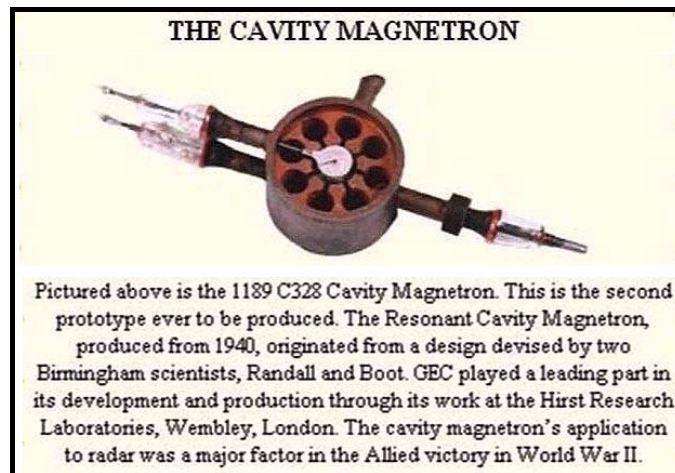
Fig. 6 - Cutout of the GEC page created around the early eighties about their cavity magnetron. It shows the eight cavities sample number 2, identical to our sample, so confirming our reconstruction [*P09].
