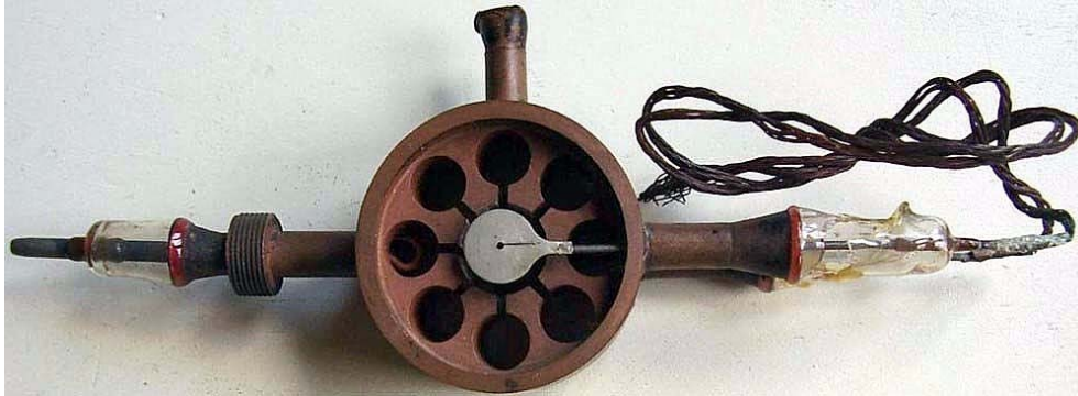
Fig. 1 - This GEC 1189 C328 is the very early eight-cavity laboratory prototype, recently found and today preserved in the ase-museoedelpro collection. [*TM-01]
