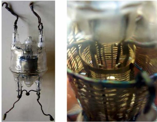
Fig. 7 - The experimental CV14 for VHF operation
