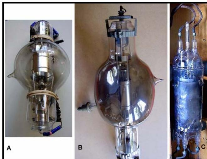
Fig. 1 - Early transmitting tubes: in A the 250 W VT30, in B the 600 W MT9A and in C a 2 kW silica triode.
